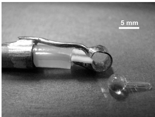
Fig. 2. Photo of the single turn solenoid coil employed. A heavily GdCl_3 doped water drop ( T_2^* , T_2 , T_1 s = 60–100 \mu s) was syringed into the bulb shown at right and flame sealed. The probe was tuned to 100 MHz and capacitively matched with a Q value of 100. The probe was enclosed in an RF shield for measurement. The probe is constructed from teflon and copper and has negligible background signal.
